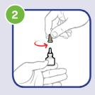
Holding the bottle upright, remove the tan cap. This will allow any excess pressure in the bottle to be released. Replace the tan cap on the bottle and close securely.
